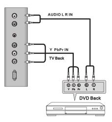
Connect the YPbPr output of the DVD or VCR to the YPbPr input on the set. The picture quality is improved; compared to connecting a regular VCR to the video input. Connect the Audio output of the DVD or VCR to the Audio input jacks on the set using the RCA cable. Select HD input source with using the SOURCE button on the remote control.
